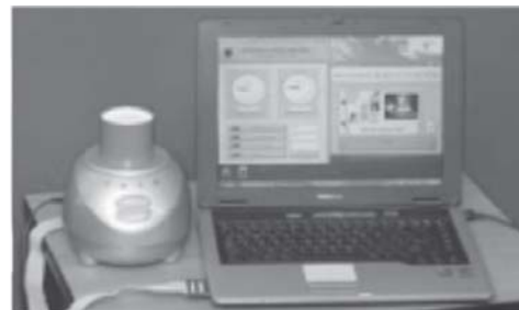
Figure 19. A prototype model for dual-frequency microwave liquid moisture meter [49].
